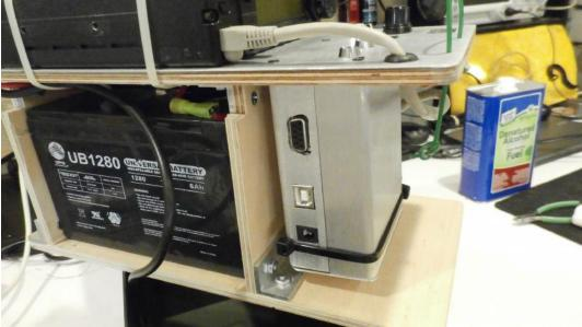
Two of the Tracker Units are built using a Byonics TinyTrack APRS units, GPS unit and BAOFENG UV-5R Transceivers.
