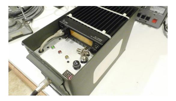
LED are used to show the state of the Digipeater, Green for On, Red for Transmit and Yellow for Received data. A LED Voltage/Current meter is installed in the enclosure. System is protected by a Fuse and a key switch for On/Off.
