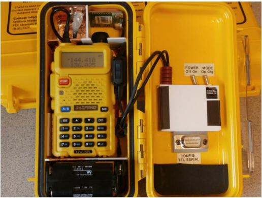
One Tracker is built with using a BAOFENG UV/5R Plus. The original 4<sup>th</sup> Tracker uses an earlier model BAOFENG transceiver (included as a Free unit. I don't need it anymore)
